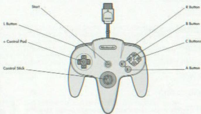
The default Controller configuration is shown here. All references to button selection in this manual refer to the default Controller configuration.
